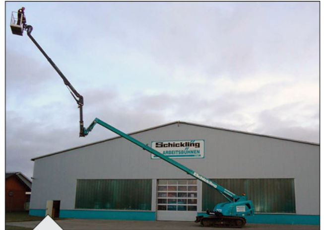
Horizontal outreach increases to a massive 26 metres with 2 persons and tools.
