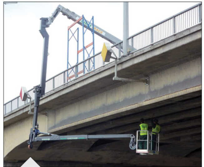
The Giraf under-bridge unit can reach up and over tall obstacles.
