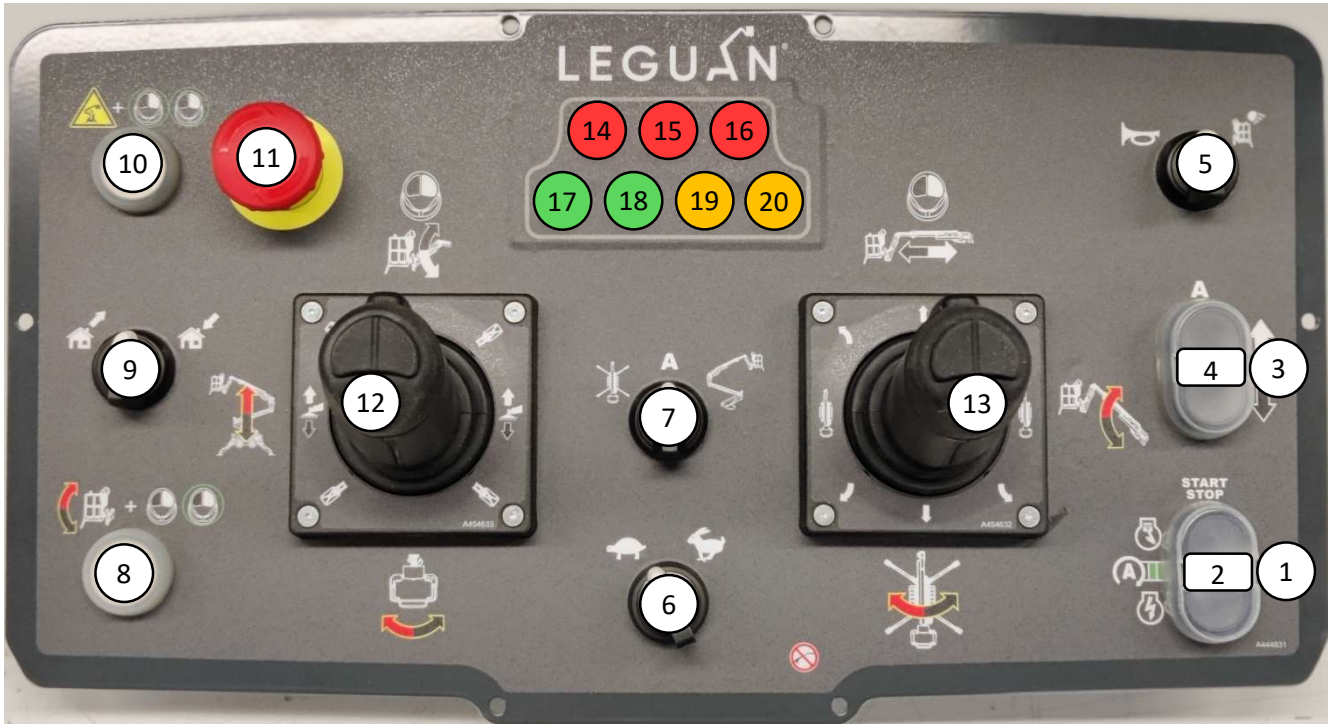
Figure 7. Platform control panel
