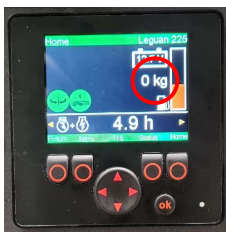
Figure 41. Work platform load on display
