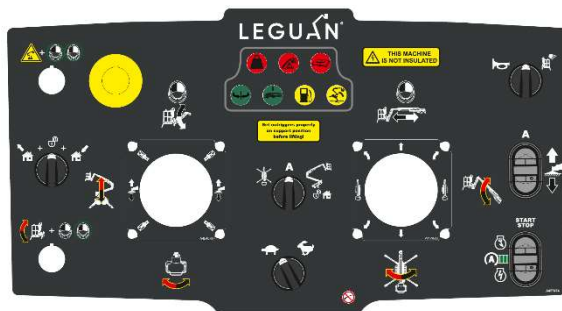
10. Platform control panel
