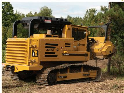
*Rayco's exclusive elevated cooling design places engine radiators in both the rear of the engine compartment and in the limb riser for maximum cooling in even the harshest environments.*
