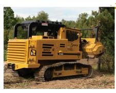
Rayco's exclusive elevated cooling design places engine radiators in both the rear of the engine compartment and in the limb riser for maximum cooling in even the harshest environments.
