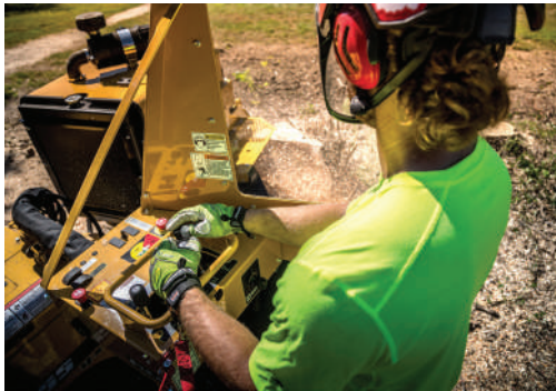
Swing-out control station protects the operator and provides the best view of the cutting action. Controls fold in line for travel through gates.
