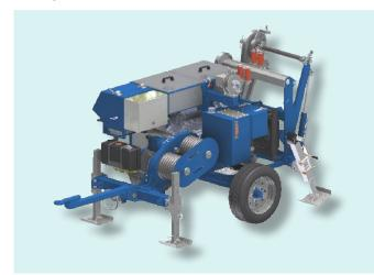
Hydraulic puller fit to pull one rope in stringing operations of overhead transmission lines. One hydraulic circuit allows to continuously vary the speed in both directions by operating one control device.
