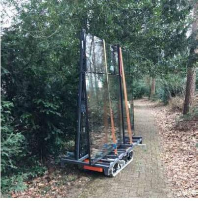
The TC1 carrier is the solution for horizontal transport of long, heavy construction material and equipment at a project site. The carrier is compact and just 80 cm wide, and material can be placed on it in the length or width. The radio remote controlled carrier is perfect for transporting material, such as steel beams, through small access doors and less easily accessible areas.
