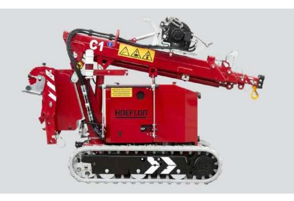
The C1 mini-crane is small yet powerful! Its compact size allows you to transport this minicrane on a trailer or in a van. The crane fits in a lift, which makes transport to an upper floor or the roof as easy as can be.
