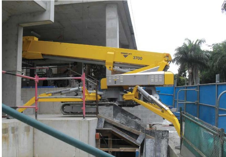
**Weighing only 5.76 t, this Omme is incredibly light for a machine that provides a huge 37 m of working height and with an increased capacity of 250kg. Horizontal outreach is now up to an impressive 13.7 m.**
