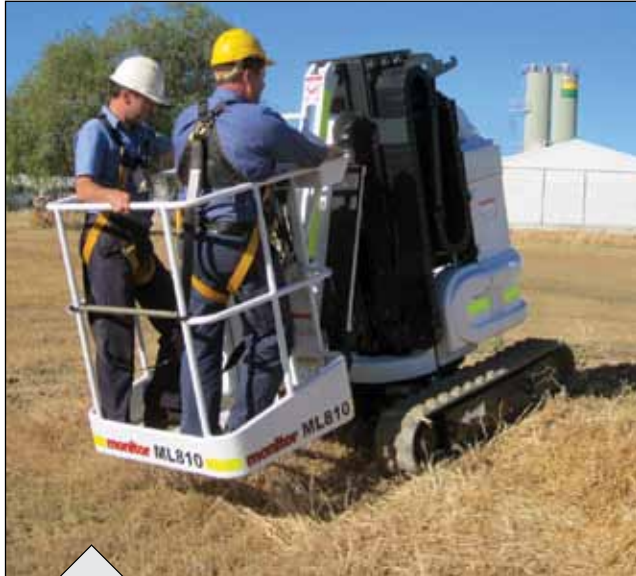
The spacious steel basket allows for two operators to work both indoors and outdoors and can safely elevate on slopes of up to 5°!
